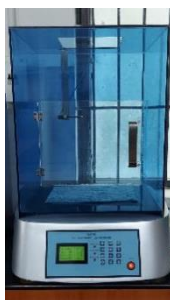
Fig.-8: Testing of thermal conductivity of nonwoven
