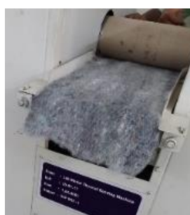
Fig.-6: Thermal bonding process
