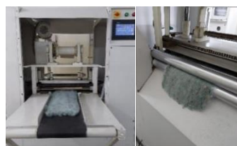
Fig.-5: Needle-punching process
